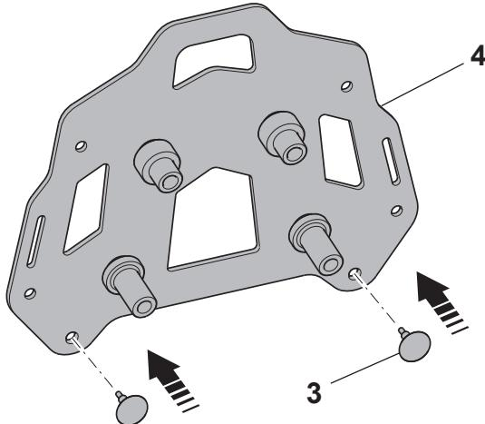
**GB** As shown in the drawing, mount the two grommets **3** on the support plate **4**.
