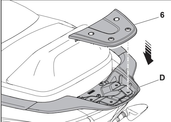
**G** Place the perforated cover **6** (supplied with the kit) on the socket of the handle **D**.
