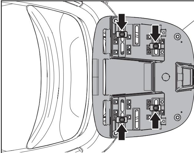
Following the directions given on the drawings, place the attachment plate 11 on the support plate with the curved brackets 12, T-bushings 13, screws (M6x20) 14, washers 15 and self-locking nuts (M6) 16.
