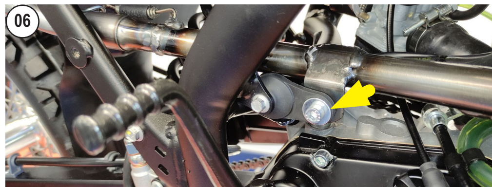
SCREW AND FIT THE MUFFLER (fits with STOCK OR LeoVince)
